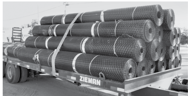
IMAGE 2: Storing the Tensar Geogrid rolls horizontally.
